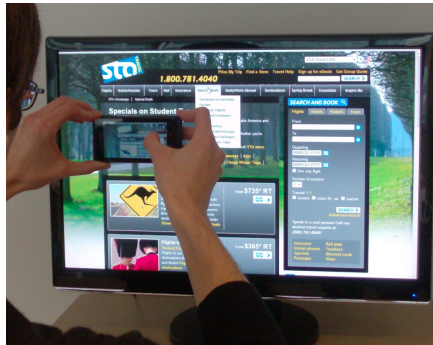
Fig. 1. A user controls the display by touching captured sensitive screen areas.
