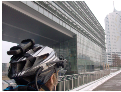
Fig. 2. A smartphone with all needed sensors is mounted at the helmet.
