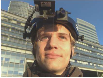
Fig. 1. The used eye tracker includes an eye camera and a scene camera.
